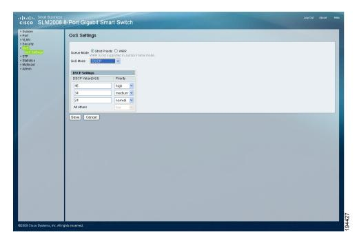
DSCP Settings—DSCP Settings enable mapping DSCP values to specific priority levels. The default DSCP settings are shown in the following table:
