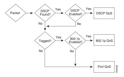
802.1p—802.1p QoS Mode allows you to specify data packet priority based on the 802.1p value in VLAN priority tag of the packet. Users can map 802.1p to one of 4 priority queues.
