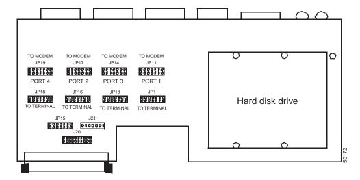
Seven jumpers are installed at jumper locations JP1, JP11, JP13, JP14, JP16, JP17, JP18 and JP19, connecting pins 1-2, 3-4, 5-6, 7-8, 9-10, 11-12, 13-14 as shown in Figure 4-9.
