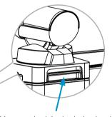
You can lock/unlock the back cover by lifting this handle. Use both hands if required.
