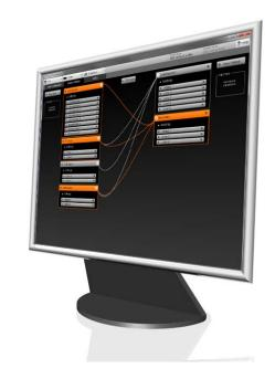
The Audio console helps you configure the audio system of the codec. It will allow you to change the default mixing, routing and equalization as well as allow you to set various input and output connector properties.
