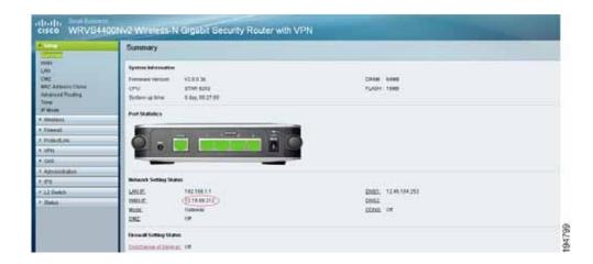
Now you should be able to access your camera over the Internet by typing in the WAN IP address of your router, a colon, and the defined port number in the following format: http://router's WAN IP address:port
