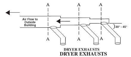
Area of section "A-A" must be equal to the sum of dryer exhaust pipes entering multiple exhaust pipe. (*See chart below*.)
