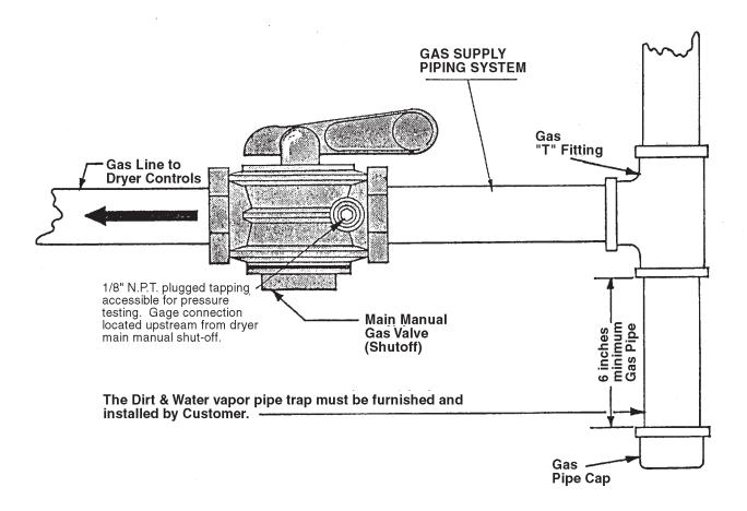
The dryer and it's individual shutoff valve must be disconnected from the gas supply piping system during any pressure testing of that system at test pressures in excess of 1/2 PSIG.
