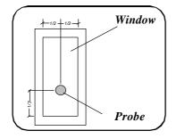
The tilt switch is mounted on the solid part of the machine. There is a window around the probe of the tilt switch that is mounted on the movable part of the machine. When the machine goes out of balance by overloading or uneven distribution of the linen, the tilt switch will interrupt this action to prevent damage to the machine.
