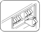
Take the necessary soap compartments out of the soap dispenser and fill them with the required detergents in function of the chosen program. Then put them back into the soap dispenser, leaning against the axle of the drop valves. See instruction manual PS 40 : "6 : Operating mode".
