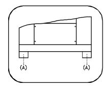
The machine must be placed on a flat, solid surface (metal base, concrete or solid ground). It is *recommended that the machine be anchored* (M16) on the provided places (A) in the base, especially in case of a plinth (see Dimensions 2).
