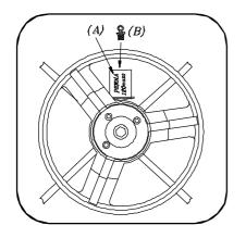
The bearing house of the machine is equipped with a lubricating device (A) which automatically lubricates the bearing during one year. Upon delivery of the machine, this lubricator has not been brought into use. To this effect, please put on the matching screw (B) in the foreseen opening of the lubricator.
