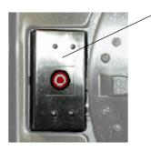
To open the door in case of emergency (malfunction, etc.), remove the lock cover plate (A). Subsequently,
