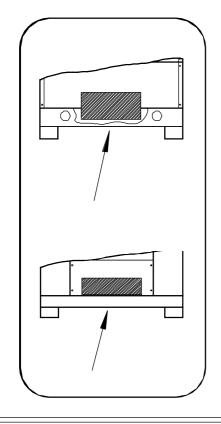
To prevent damage during transportation, the machine has been equipped with *four red transport brackets* (D) to eliminate every possible movement of the tub. After the machine has been placed level, take off the service- and the back panel to remove these transport brackets.
