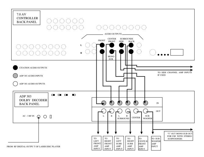
If you are using the side channel outputs of your Citation 7.0 controller, leave these channels connected directly to the side channel amplifier inputs. These channels will not be used for Dolby Digital playback of the ADP 303 digital processor. They will, however, still be used for all playback of 2 channel modes such as 6 AXIS, 70 MM, Dolby, and THX.
