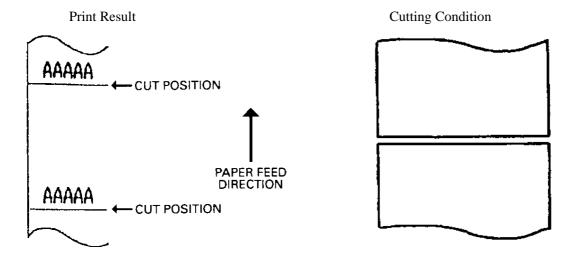
(42) Partial Cut (ESC m) (In selection of cutter option)
