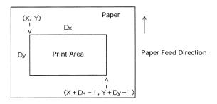
The printable area for this printer is approximately 72.070 mm (576/203 inches) horizontally and 117 mm (1662/360 inches) vertically.
