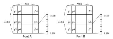
Create each data bit by setting "1" for a printed dot and "0" for an unprinted dot.
