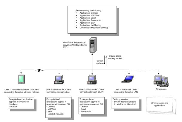
This is a diagram showing multiple users of MetaFrame Presentation Server Clients on a variety of devices, which are connecting to a server farm and accessing published applications and resources.
