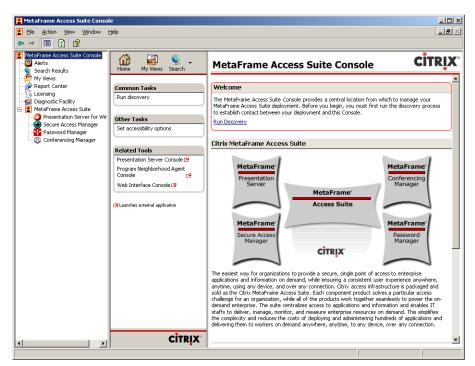
This screen capture shows the Access Suite Console before running discovery and with the MetaFrame Access Suite node expanded.
