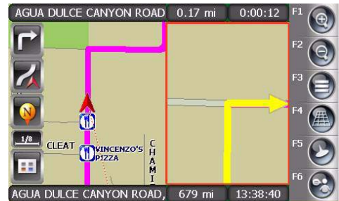
Enlarged intersection on the right
