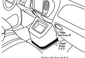
Position L-Brackets attached and mark transmission hump locations
