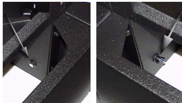
Side-to-side bolt with wing nut at bottom of neighbor Margays
