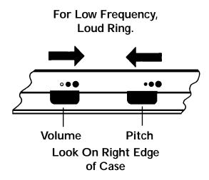
The Ringer Volume Control has three settings: OFF, LOW, and HIGH. It is suggested that you set the volume control to high when you first start using your Walker Clarity. To do this, slide the ringer volume control toward the largest dot.
