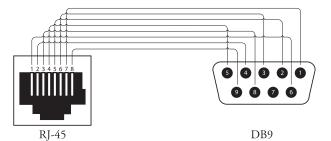
Remarks: The Cat 5 cable and connector that is used for the adaptor and plugs into the rear panel RJ-45 port must use pin-to-pin wiring.
