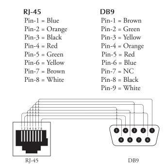
Remarks: The Cat 5 cable and connector that is used for the adaptor and plugs into the rear panel RJ-45 port must use pin-to-pin wiring.
