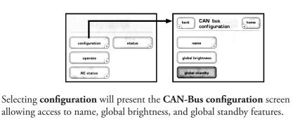
*operate* The **operate** settings allow you to bring the target unit in and out of standby, or mute. This key will be disabled for the unit whose touchscreen you are using to access CAN-Bus.
