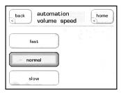
This volume control is specifically for use with automation control systems. Such control systems can vary in how quickly they repeat ramped volume commands. By first selecting a suitable volume control speed on the SSP-800/CT-SSP Surround Sound Processor, the programming required to tailor the speed from the control interface is simplified.
