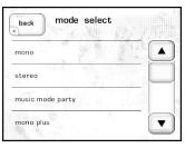
Touching the **up** or **down arrows** scrolls through the list of modes. Touch any mode (that isn't grayed out) to select it. The SSP processing changes to the newly-selected mode. Press the **Back** button to return to the Home page. The available modes are described in Table 2.
