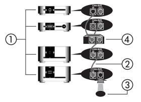
NOTE: Daisy chain must be terminated with CAN-Bus Terminator.
