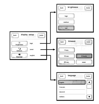
This button brings up the **display setup** menu. It allows you to configure the CP-500's LCD screen *brightness*, the display *timeout*, and the *language* used in the touchscreen and menu system.
