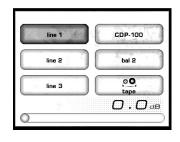
When an input is renamed 'SSP', it becomes a unity gain input. When such an input is selected, the volume control of the CP-500 is disabled, all outputs are driven at line level and the volume indication is removed from the main menu.
