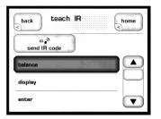
The CP-500 provides discrete infrared (IR) command codes for all its functions, a list that extends far beyond what is required by normal remote controls. However, many of these functions are critical if you plan to create a customized remote control with macros that take command of your entire system. Without these discrete codes, many of the macros you might want to create will simply not work reliably.
