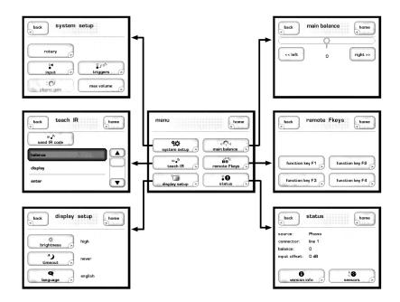
Pressing the front panel **Menu** button to the left of the **LCD touchscreen** brings up a comprehensive *main menu system*, the top two levels of which are shown above. This menu provides access to many installation-specific features that let you customize how the CP-500 works within the context of your particular system.
