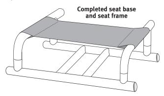
Locate the seat base and find the curved legs. With the curved legs to the front, insert the seat platform rails onto the pontoon frame posts. (The front of the pontoon frames are the ends labeled "L" and "R").
