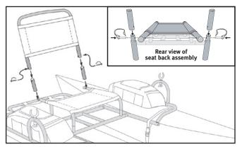
Slide the seat stubs onto each end of the seat back frame. Next, slide the seat back panel onto the seat back frame. Then place the assembled seat back into position on the outsides of the seat frame and secure to the seat base with the two long clevis frame pins.
