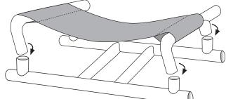
If you can't press the seat platform into the seat frame you can turn the assembly upside down (so that the fabric is on the ground) and stand on the seat rails. You can also use a rubber mallet.
