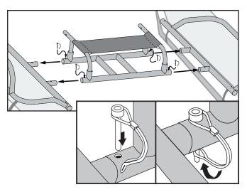
**7. Insert the foot pegs.** Locate the front of the pontoon frames, (the end
