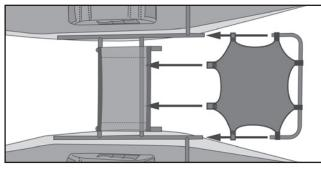
the front of the cargo deck frame into pontoon frames. Insert a short clevis frame pin on either side of the frame from the top down into the holes where the cargo deck frame slides into the pontoon frames.
