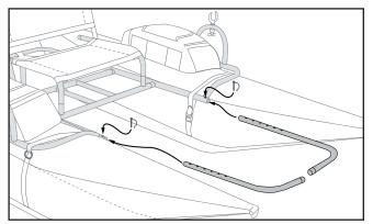
the pontoon frame and attach with short clevis pins. Choose a position in the middle of the adjustment range.
