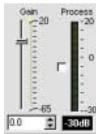
Figure 3.57. Process gain adjust and meter
