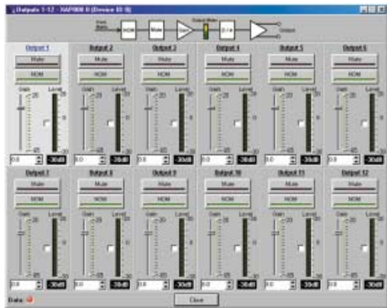
Figure 3.48. Outputs 1-12 configuration window
