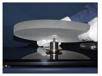
Place the pulley on the motor spindle. The distance between the pulley and the motor housing should be approx. 1-2mm. Tighten the little screws inside the pulley with the aluminium screwdriver provided.
