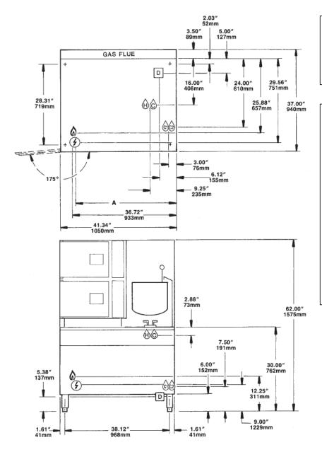
NOTE: When ordering optional reverse door openings: Control Panels, door openings, cooking compartments, clearances, and kettle are opposite that shown.
