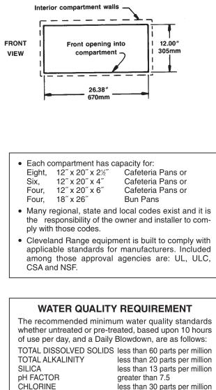
Consult a local water treatment specialist for an on site water analysis for recommendations concerning steam generator feed water treatment (if required), in order to remove or reduce harmful concentrations of minerals. The use of highly mineralized water will mean that more frequent servicing of the steam generator will be necessary. The fact that a water supply is potable is not proof that it will be suitable for the generator.
