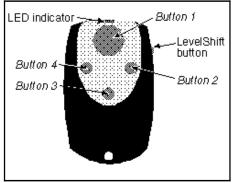
of the remote control allows you to select channels 5–12:
