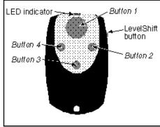
on the side of the remote control allows you to select channels 5–12:
