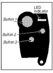
Your 3-Button/3-Channel Remote Controls The 3-button/3-channel keychain remote control is a sophisticated radio transmitter that sends unique digital
