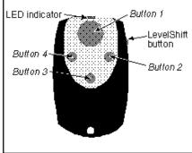
*within the next 7 seconds*. For instance, to transmit channel 5, press the LevelShift button once, then press button 1. While you transmit, you'll notice that the LED indicator blinks twice, pauses, blinks twice, etc.: this indicates **level 2**.
