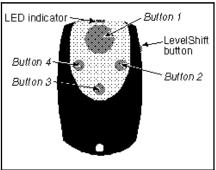
■ To transmit either channel 1, 2, 3 or 4: Just press either button 1, 2, 3 or 4.
