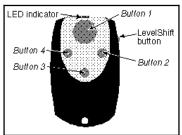
■ *To transmit channel 9, 10, 11 or 12:* Press LevelShift twice to shift buttons 1–4 to level 3 (channels 9–12), then press the corresponding button. Thus, to transmit channel 10, press LevelShift twice, then button 2. You'll notice that the LED flashes three times, pauses, flashes three times, etc.: this indicates **level 3.**
