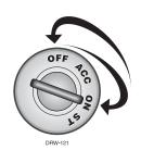
Turn ignition to "on" position, turn to "off" position. Press and release the integrated LED/Valet® switch within 10 seconds. The status LED will
