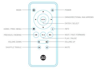
NOTE: Volume controls are not available while using an HDMI cable. You must control volume with your TV or home stereo remote control.
