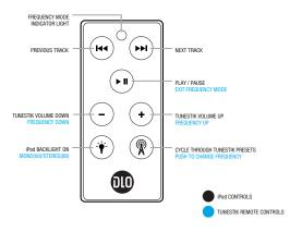
The TuneStik is a "mini" radio transmitter that broadcasts your iPod audio through the FM radio in your car. The TuneStik features a powerful RF Remote Control that easily attaches to your steering wheel so you can control your iPod playback and navigation without taking your hands off the wheel. It can also be used to play your iPod at home, in a hotel, at a friend's house – anywhere there's an FM radio nearby.
