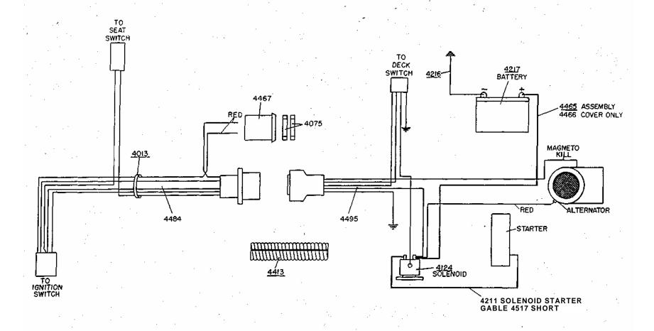
BODY WIRING LOOM - 4484 REAR WIRING LOOM-4495 WIRING KIT (308-311)-8669 (SEE ASSEMBLY BREAKDOWN) Free Manuals Download Website
