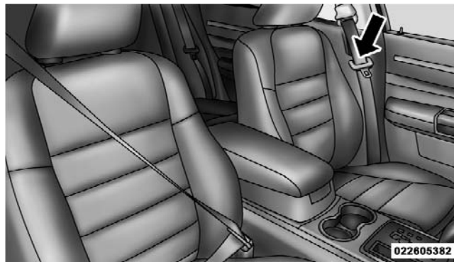
Pulling Out the Lap/Shoulder Belt Latch Plate
