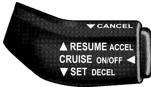
Electronic Speed Control Lever
