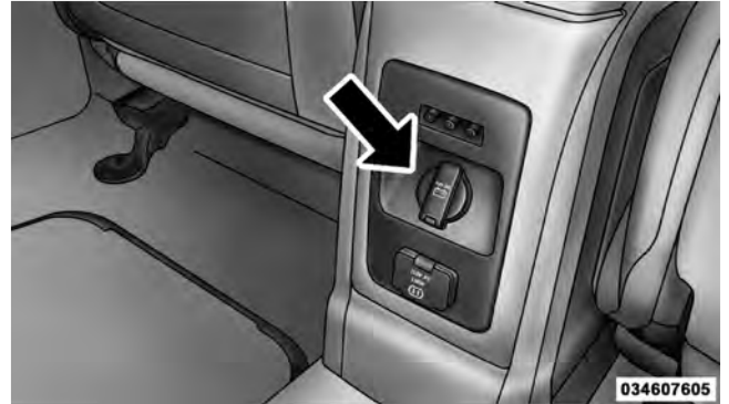
Rear Power Outlet
