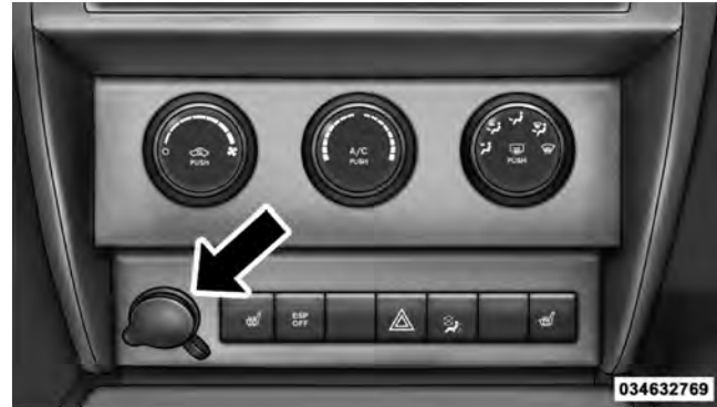
Front Power Outlet
