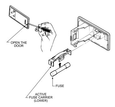
Check that the fuse in the active (lower) fuse carrier is of the correct rating. A spare fuse can be stored in the upper fuse carrier position.
