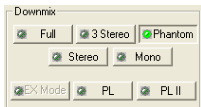
Figure 5-3 Downmix Monitoring Controls
