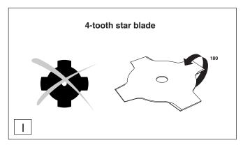
Note: The cutting tools below should be sharpened <u>only</u> at a qualified <u>workshop!</u> Manual resharpening will result in an imbalance of the cutting tool, causing vibrations and engine damage.
