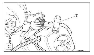
Insert the wrench (C/7) between the housing and the cylinder, only as shown in the illustration.
