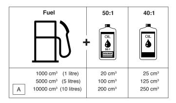
The brushcutter is powered by a high-performance two-stroke engine. The engine runs on a mixture of gasoline and two-stroke engine oil.
