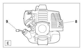
The felt filter (E/9) of the suction head is used to filter the fuel taken in by the carburetor.
