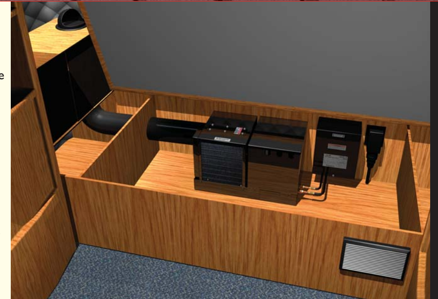
Split system inside unit beneath bunk.
