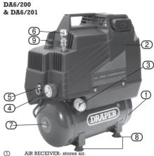
MOTOR COWLING- covers, protects hot/moving parts.
