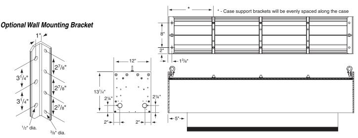
\*Please Note: Optional wall brackets add 1¾" per bracket to case length. Wall mounting bracket hole location is 1" from end of case.
