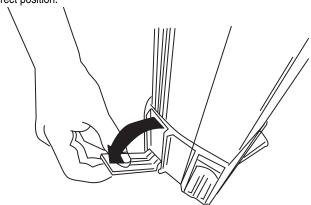
② Place closed unit with carry handle on left side (from audience perspective). Depress two buttons on front and back of housing (clearly marked) with thumb and index finger. Open screen slowly to desired width.
