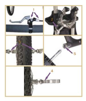
Replace the brake pads when the grooves become worn away. Check all bolts are tight and springs are secure for rear foot brake.
