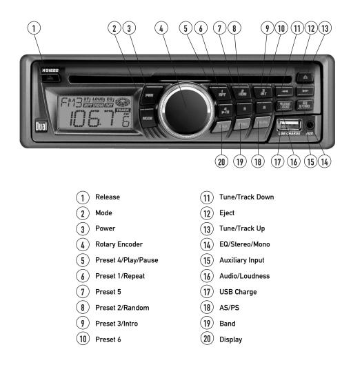
The XD1222 has an easy-to-use interface that provides a rewarding experience, as well as support for your favorite tunes. Audio CD-R and CD-RW disc playback ensures compatibility with your music collection, and the RCA preamp output provides the right connections to expand your system. From its front panel auxiliary input for connecting your MP3 player, to the detachable face for security assurance, this head unit has you covered.
