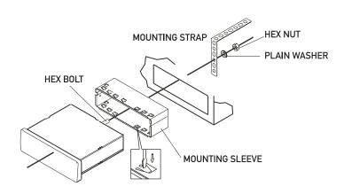
TYPICAL FRONT-LOAD DIN MOUNTING METHOD
