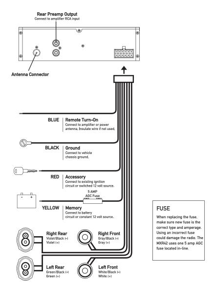
\* Caution - Do not attach any speaker leads to ground as severe damage will occur.
